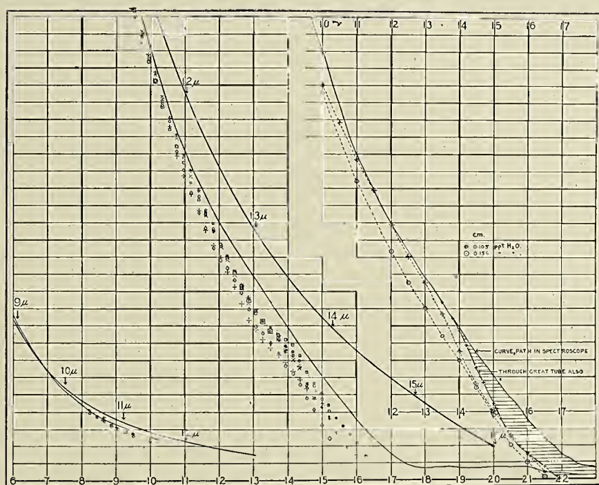
FIG. 40.—Energy curves showing absorptions produced by water vapor, 15^\circ rock-salt spectrum, 9 to 17\mu .
